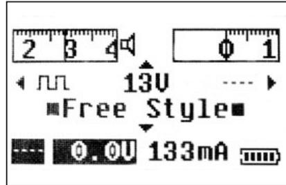
This screen shows that an LNB is connected on the left; polarisation is vertical (13V setting), 22kHz tone is on, and the speaker is on for audible signal strength.
